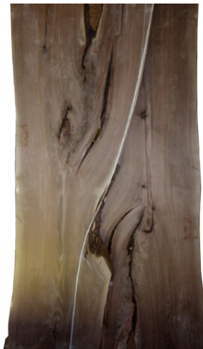
Curve joining is when two slices of the same tree are joined along a natural curve.
